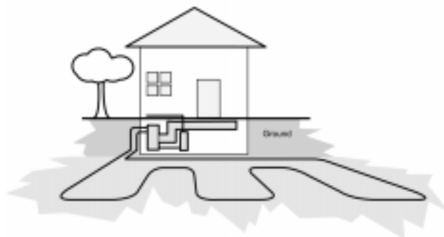
FIGURE 1 Residential GHP system
